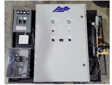
On-Site Oxygen Generator
